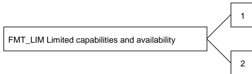
FMT\_LIM.1 Limited capabilities requires that the TSF is built to provide only the capabilities (perform action, gather information) necessary for its genuine purpose.
